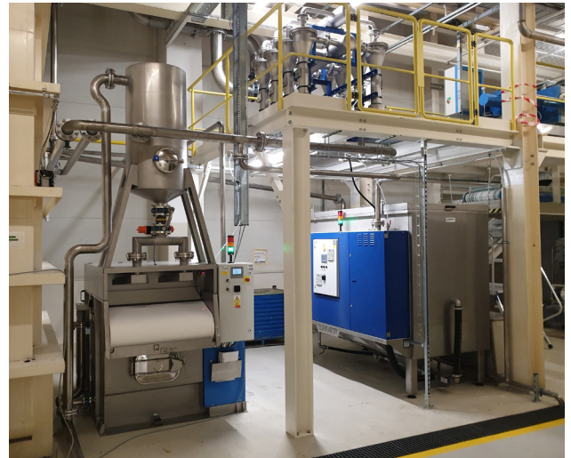
A typical bath maintenance setup for pretreatment in an automotive paint line with Suparator® and Q-Filter®.
