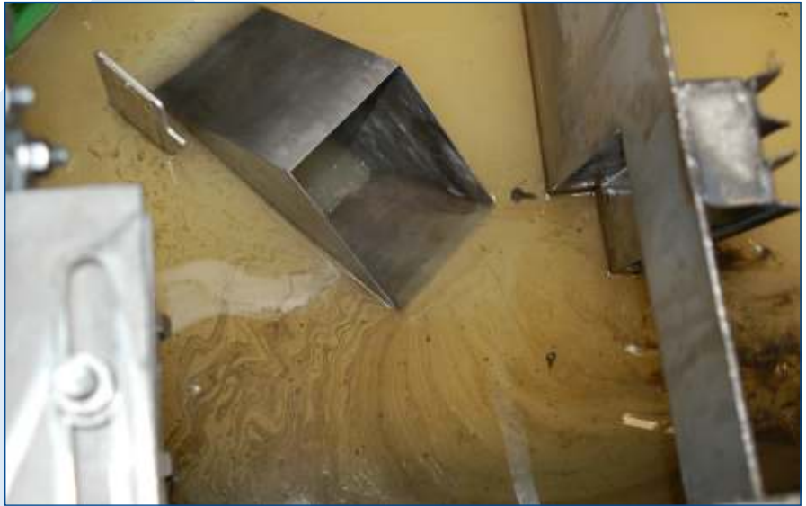
A Suparskim® skimmer in action, mounted in the clients washer tank. Any oil is automatically and immediately carried off with the flow.
