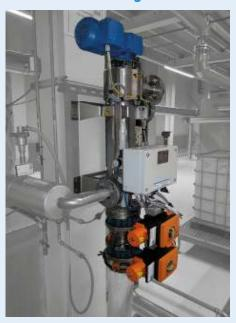
Q-Mag<sup>®</sup> automatically removes metal particles from a medium. The medium spirals around the rotating magnet, which significantly increases the chance that fines will be attracted by the magnetic field. The result is an extremely efficient separation of even the finest magnetisable particles.
